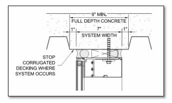
22) If anchoring to underside of a composite concrete slab, the corrugated decking needs to stop where the Talon Wall units are located, and a full-depth slab is required. This is to avoid the anchor bolts occurring at the high point of the corrugated decking, as well as providing a consistent sealant surface.
