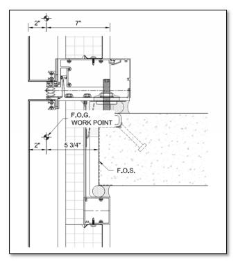
4) If a thicker infill is used, for example a protruding metal panel, the 5 ¾" dimension to Face of Slab is still from the theoretical Face of Glass (this can also be referred to as the face of system workpoint). The protruding infill will extend out beyond this workpoint.
