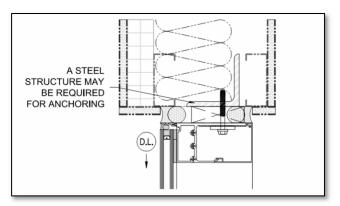
10) When anchoring a unit at an overhang condition that has a drop ceiling, keep in mind that Talon Wall is dead loaded at the head. This means the substrate being anchored to needs to be robust enough to handle the weight of the unit. It's not uncommon for the substrate of a dropdown ceiling to just be shown as a metal stud framing system, which may not be adequate.
