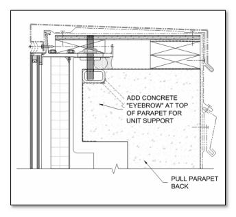
14) Where large concrete parapets occur, it is recommended to explore with the design team if the parapet can be pulled back, with a concrete "eyebrow" added at the top of the parapet that mimics a typical slab edge condition. This allows the mullion notch-out to be minimized, and avoids custom embeds or steel structure.
