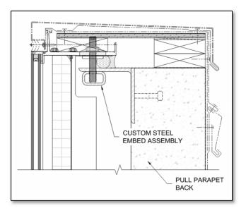
15) Where large concrete parapets occur, and Item 14 cannot be accommodated, the next best solution requires pulling the concrete parapet back and using a custom embed assembly at the top for unit anchoring. The steel angle should be continuous in order to provide a sealant surface. The steel tube below is only required at mullion locations.
