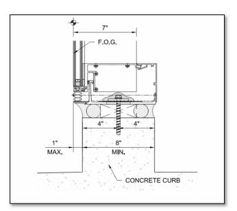
7) If a starter track occurs at a curb, the face of the curb should be flush with Face of Glass, or at maximum, located 1" behind Face of Glass and a sweeping sealant joint can be utilized. The concrete curb width should also be at least 8" to achieve the minimum edge distance required for the anchor fasteners.
