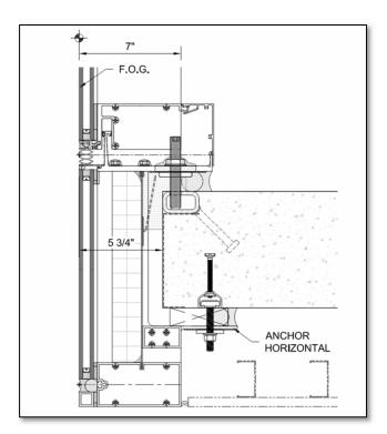
16) If a project requires "slab edge cover" units, this can be accomplished by using the custom horizontal member that allows for supplemental anchoring at underside of slab. There is a limit to how far the unit can cantilever down past bottom of slab, which will vary per project loads.
