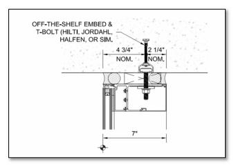
9) When anchoring a unit at underside of slab, such as at balcony conditions, a typical embed channel and T-Bolt will be used from a manufacturer like Hilti, Jordahl, Halfen, or similar.
