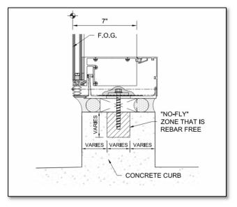
8) At concrete that is not post-tensioned, such as curbs, where drilled concrete anchors are used, a "no-fly" zone should be coordinated that provides a rebar-free area at anchor locations. The size of the zone will vary per project anchoring requirements, but the location of these zones will generally be located roughly 4" to the left & right of each mullion.
