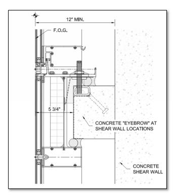
12) Where concrete shear walls occur, it's recommended to explore with the design team if an "eyebrow" can be added to the face that mimics the adjacent concrete slabs. This allows for consistent and typical embed placement. If this cannot be accommodated, a custom steel support structure will be required.
