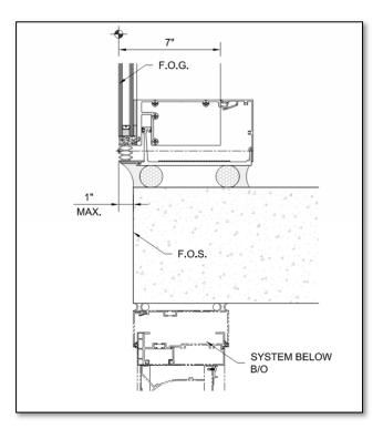
6) At starter track locations, Face of Slab needs to be flush with Face of Glass, or at maximum, located 1" behind Face of Glass and a sweeping sealant joint can be utilized.
