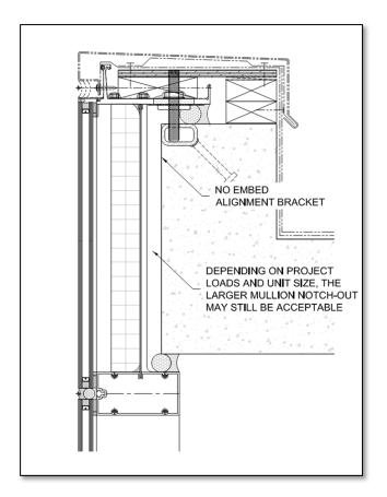
13) Where concrete parapets occur, and the height of the parapet is minimal, a typical unit configuration may still be acceptable depending on the loads of the project and the size of the unit. This will result in a larger mullion notch-out, which as noted previously will likely require mullion reinforcing and even supplemental anchoring at underside of slab. Note at these locations, the embed assemblies will not come with alignment brackets, since they would be large and unwieldly.
